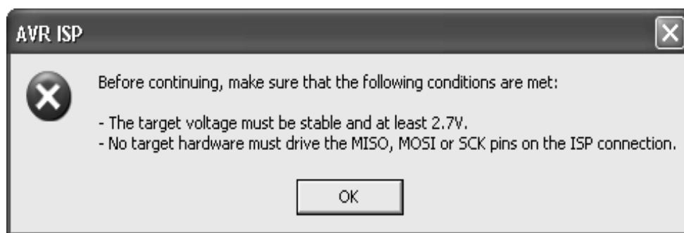
Figure 8-2 target voltage warning
