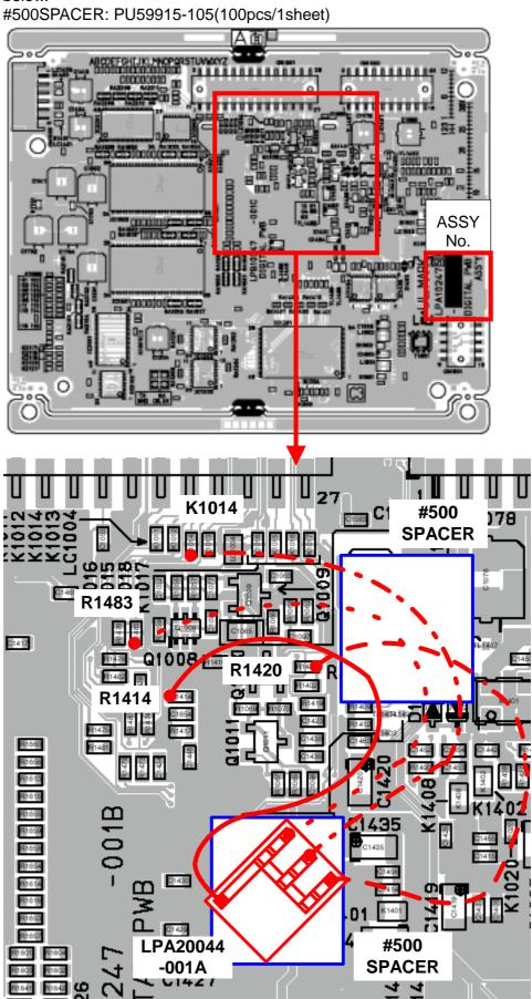
C) Add a SUB PWB ASSY (LPA20044-001A) on the DIGITAL BOARD ASSY as shown below.
