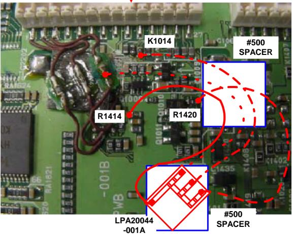
B) Add a SUB PWB ASSY (LPA20044-001A) on the DIGITAL BOARD ASSY as shown below.
