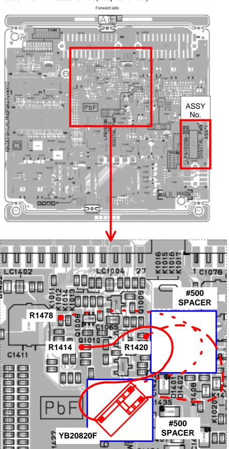
B) Add a SUB PWB ASSY (YB20820F1) on the DIGITAL BOARD ASSY as shown below. #500SPACER: PU59915-105(100pcs/1sheet)
